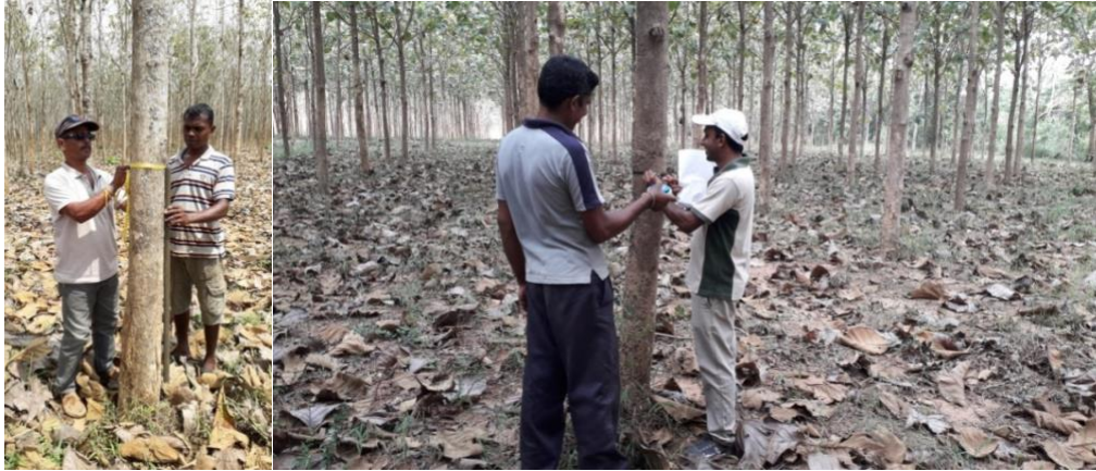
Figure 2.2. Diameter at breast height (1.3m) is measured by diameter tape. (left Anamaduwa- Right Puttalama). Inventory team follows all the standard and rules recommended in this regard.
